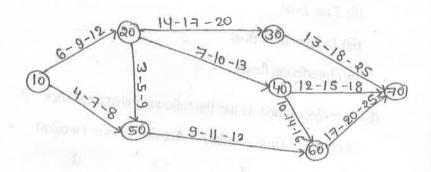
(d) In the PERT network shown in fig. the activity time estimates (in weeks) are given along the arrows. If the scheduled completion time is 23 weeks, calculate the latest possible occurrence times of the events. Calculate the slack for each event and identity the
